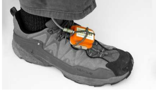
Figure 5.3: The orange XSens motion sensor is held on by the shoe laces [17].
